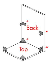
Install the back panel using the rivets with the same method as in step 2.
