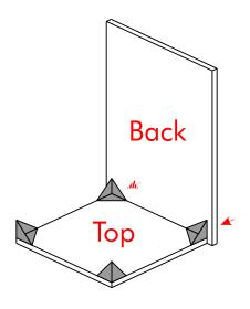
Install the back panel using the rivets with the same method as in step 2. The back sheet is slightly bigger than the side panels.
