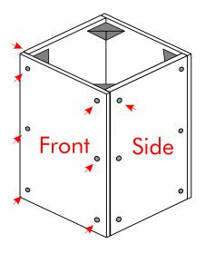
Install the front panel using the rivets with the same method as in step 2.
