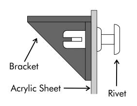
Align the holes in the bracket with the holes in the top acrylic panel.
