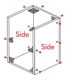
Install the side panels using the rivets with the same method as in step 2.
