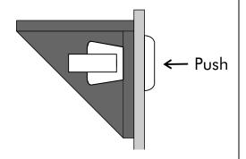
Push the head of the rivet as far as it will go. It should completely rest against the acrylic.
