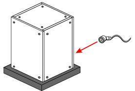
Connect the included magnetic power cable to the LED Base.
